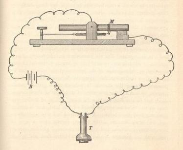
acts as an axis, and makes it into a lever. On the board he places another smaller piece of carbon similarly treated, and upon this rests another similar sized piece of carbon, the two being connected by a piece of paper. (See Fig., in which M represents the transmitter, B the battery, and T the telephone.)
