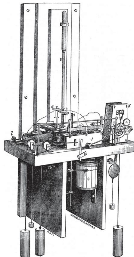
Figure 2. Line-drawing of a barograph by W.E. Knowles Middleton, from *The History of the Barometer*. (© Baros Books, Trowbridge, Wilts.)
